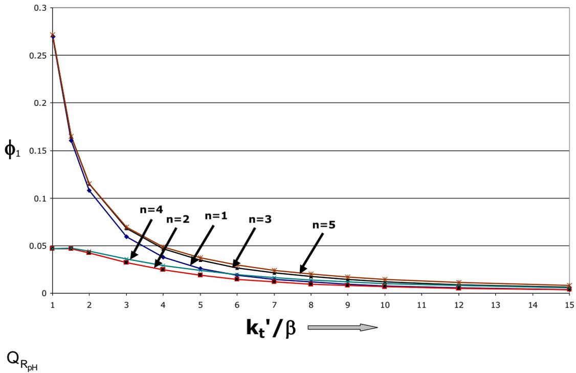
Figure 1a  $\hat{\phi}_1 = \hat{I}_{R_{pH}}^2 \beta / v^* \Delta pH$  vs.  $k'_t / \beta$  plots of the first five allowed solutions,  $n$ , from Equation I-8a and the definition of  $x$  for a given  $y$  (starting at  $y=1$ ).
