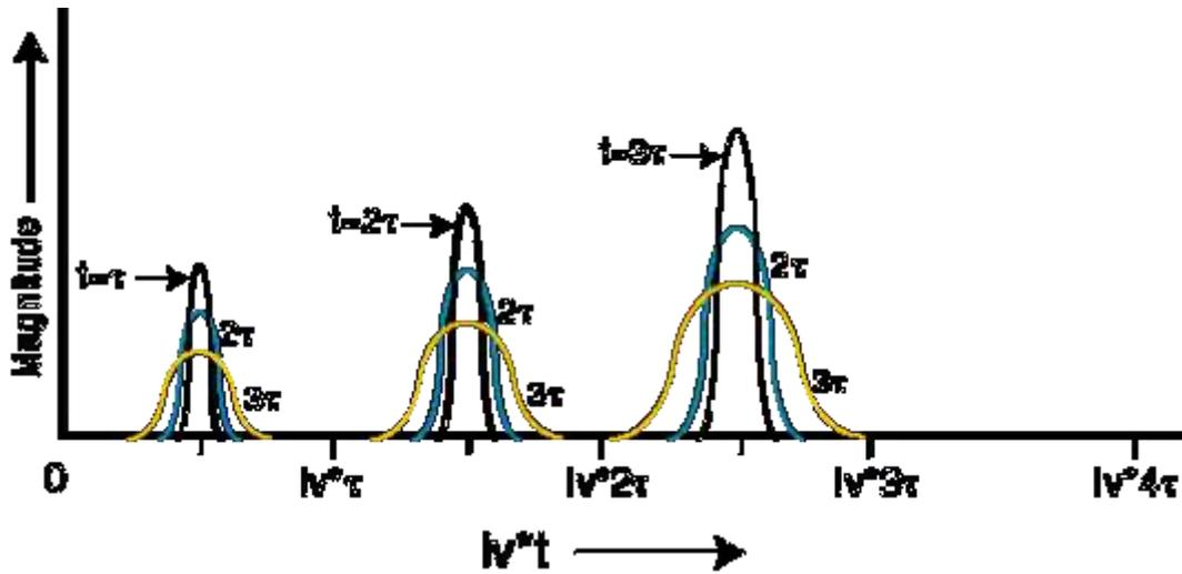
Figure 4. Gaussian-shaped phantoms generated during each pH measurement cycle.
