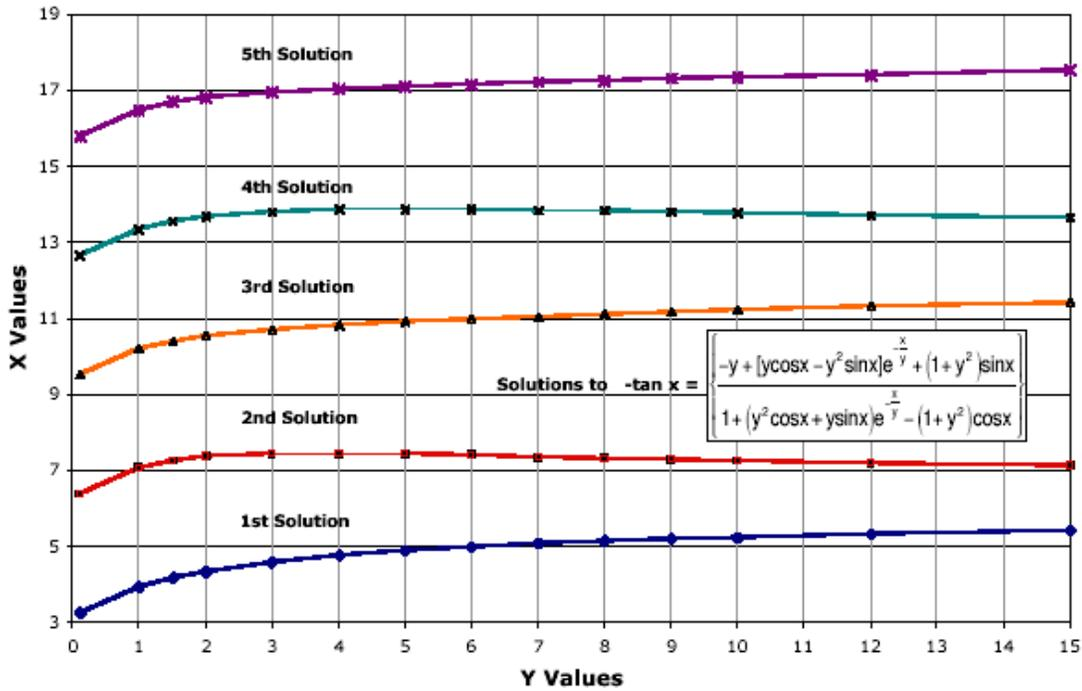
Figure Ib. Multiple solutions for  $x$  as a function of  $y$  from Equation I-8a.
